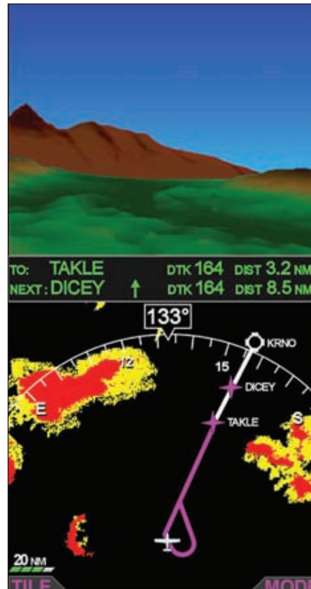
Aspen's view of the future includes detailed terrain display, left, and synthetic vision based on data derived from a three-dimensional terrain database, right. These features will be available in future iterations in a version called the ATP.
