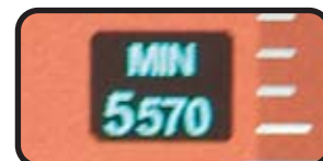
Electronic displays bring safety and workload-reducing features to the cockpit. Lateral and vertical deviation information is shown on the Aspen's top attitude display during an approach (above). The pilot can also set approach minimums as a constant reminder (right).
