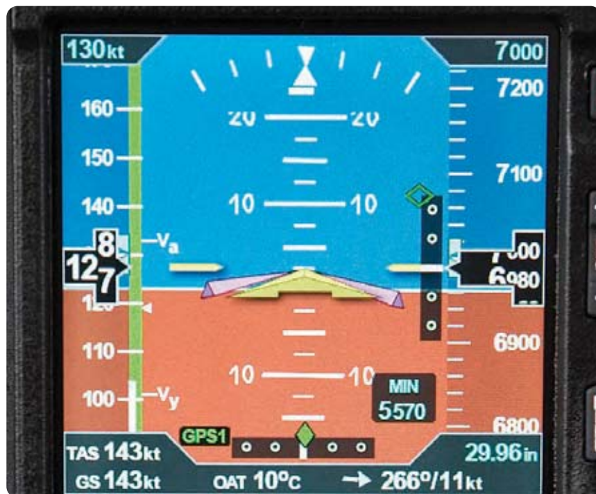
Electronic displays bring safety and workload-reducing features to the cockpit. Lateral and vertical deviation information is shown on the Aspen's top attitude display during an approach (above). The pilot can also set approach minimums as a constant reminder (right).
