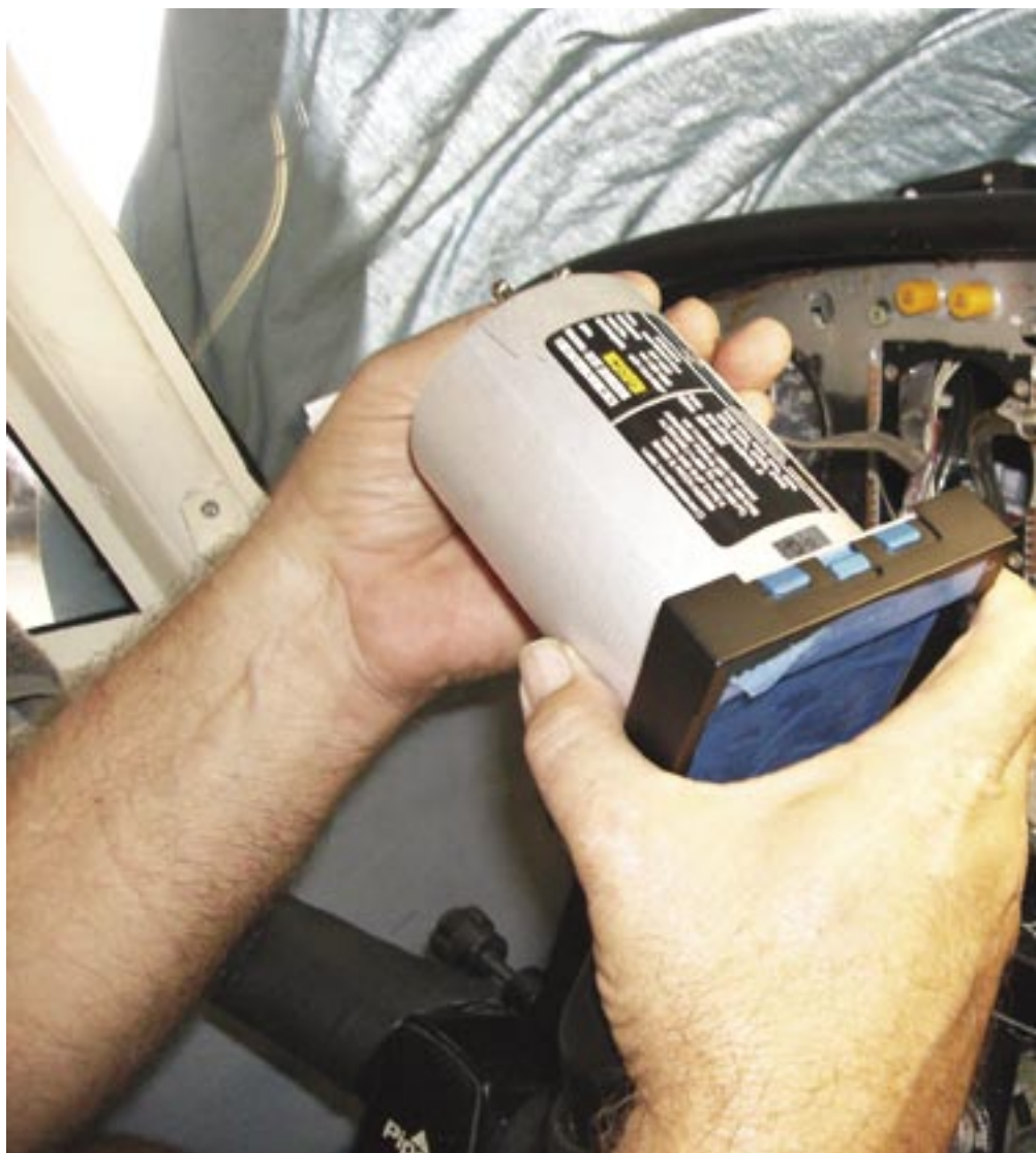
Aspen's avionics are designed to fit in the existing panel holes.
