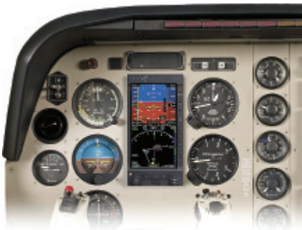
The Evolution Flight Display system is modular, allowing it to be installed as one, two, or three panels and can be expanded at any time.
