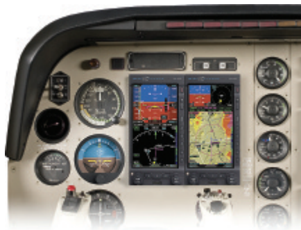
The Evolution Flight Display system is modular, allowing it to be installed as one, two, or three panels and can be expanded at any time.
