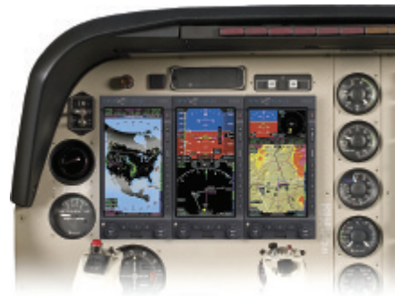
The Evolution Flight Display system is modular, allowing it to be installed as one, two, or three panels and can be expanded at any time.
